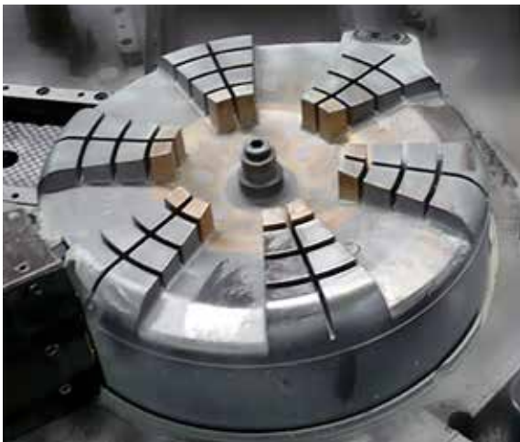
A core for moulding of washing machine drum, made of ASSAB 618 T inserted with copper beryllium.
