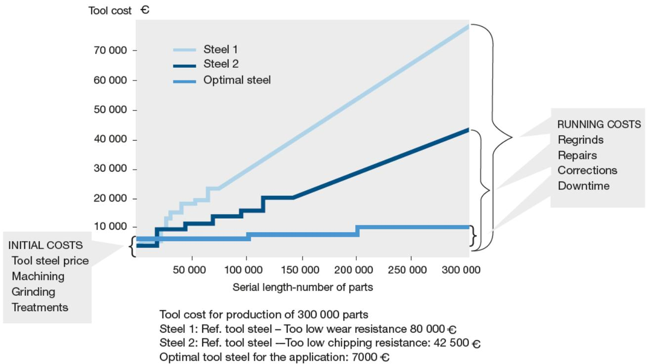
Figure 3: Total tool cost considerations. Steps in lines indicates cost for refurbishment.
