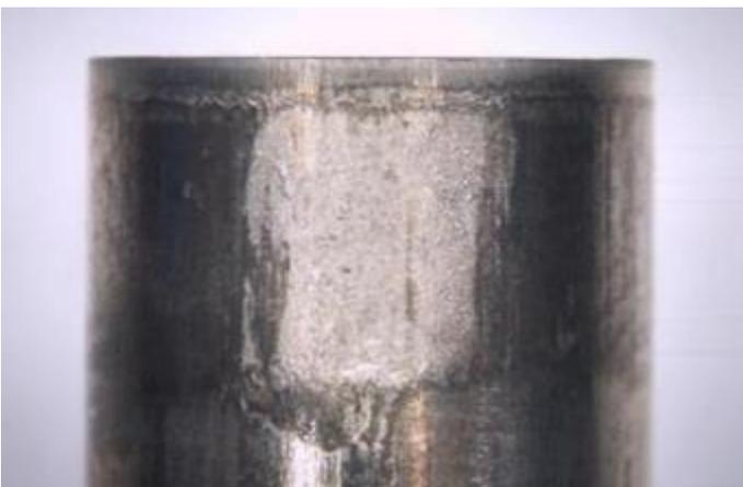
*Figure 7. Stamping punch suffered severe galling*
