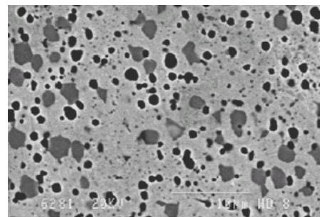
Figure 6. PM grade that contains 13% (9% MC+ 3% M7C3) mixed size carbides
