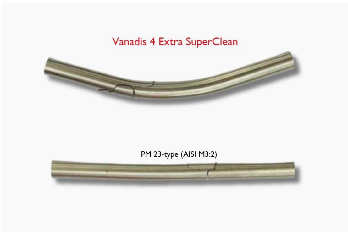
Figure 1. Four-point bend test comparison with PM 23-type, 60-62 HRC
